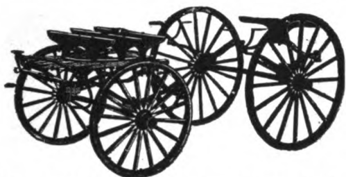
No. 60 L. Ready for body. 9 sizes— 1\frac{1}{4} to 1\frac{3}{4} in. axles.
